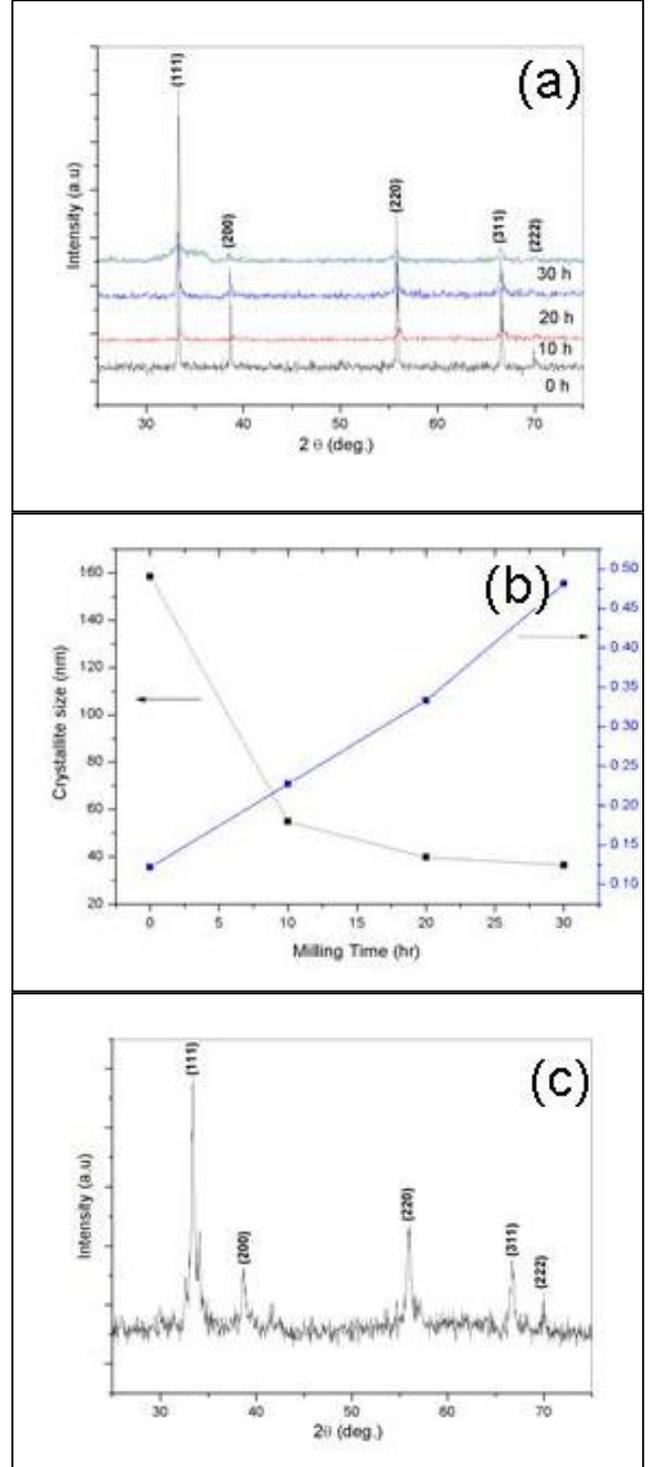
Figure 1. (a) X-ray diffraction patterns of (0, 10h, 20h and 30h) ball milled ceria, (b) effect of milling time on particle size and lattice strain of ball milled ceria, and (c) x-ray diffraction pattern for solution combustion synthesised ceria
