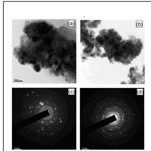
Figure 4. shows the high resolution TEM micrographs of (a), (b) ball milled and (c), (d) combustion synthesised ceria powder.
