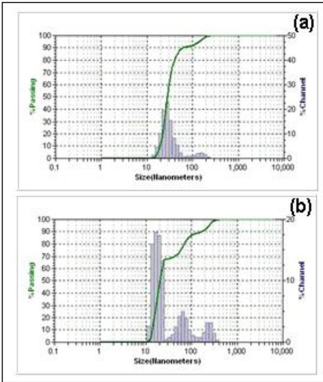
Figure 2. Particle size distributions of ceria (a) 30 hrs ball milled, and (b) combustion synthesised
