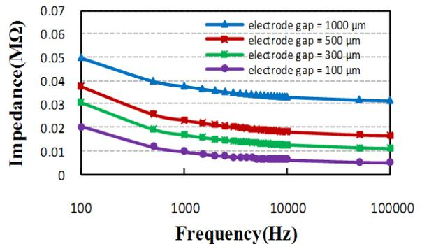
Figure 6. The magnitude of impedance according to frequency as variation of the distance of electrodes ( $A=500 \times 500 \mu\text{m}^2$ ,  $W=500 \mu\text{m}$ ).
