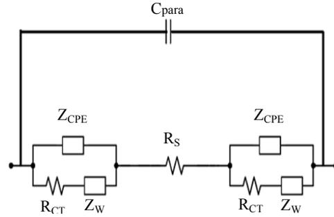
Figure 4. The equivalent circuit model for the analysis of impedance.
