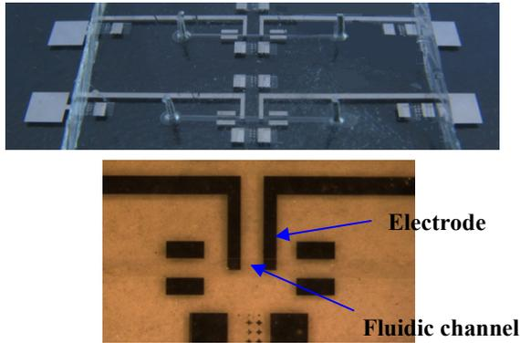
Figure 3. The fabricated chip and magnified view of the flow channel.
