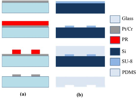
Figure 2. The fabrication process of (a) coplanar electrodes and (b) a flow channel.
