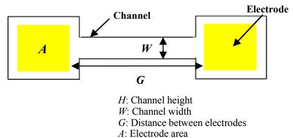
Figure 1. The schematic of sensor with coplanar electrodes.
