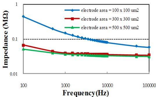
Figure 5. The magnitude of impedance according to frequency as variation of electrode area ( $G=1000 \mu\text{m}$ ,  $W=500 \mu\text{m}$ ).
