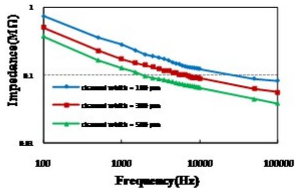
Figure 7. The magnitude of impedance according to frequency as variation of channel width ( $A=100 \times 100 \mu\text{m}^2$ ,  $G=500 \mu\text{m}$ )
