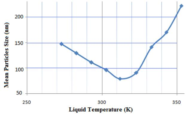
Figure 2. Liquid Temperature impact on the mean particle size
