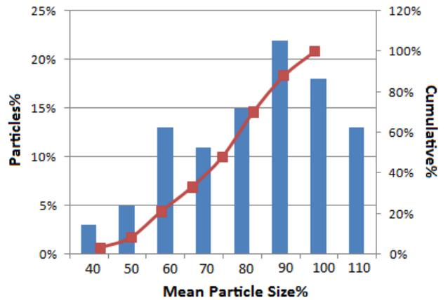
Figure 3. PSD test result for a particle with 87 nm diameter
