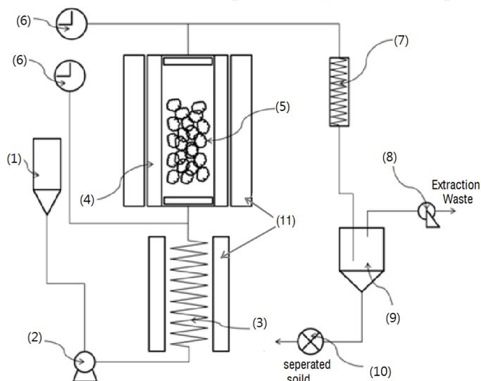
Figure 1. Schematic of superheated water extraction system. (1) Water Tank, (2) High pressure pump, (3) Preheater, (4) Extractor, (5) Soil, (6) Safety valve and gauge of temperature and pressure, (7) Chiller, (8) Back pressure regulator, (9) Separator, (10) separator valve.
