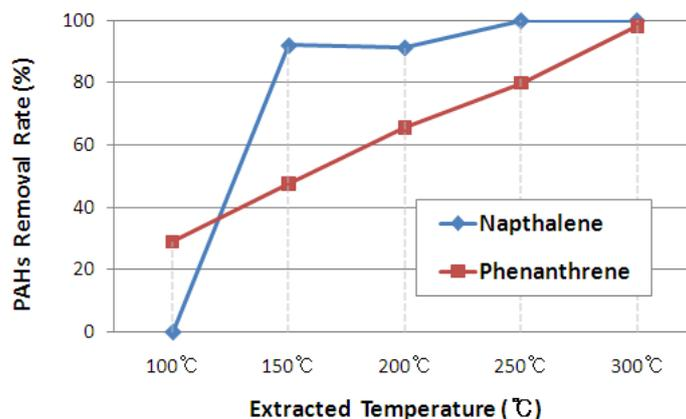
Figure 3. Removal percent of naphthalene and phenanthrene at each extraction temperature.
