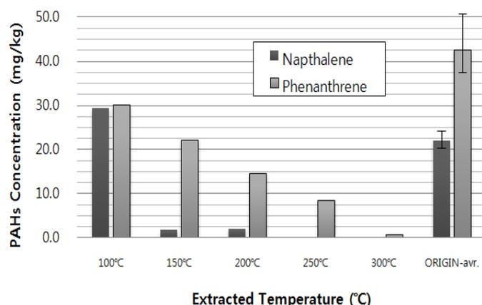
Figure 2. Naphthalene and phenanthrene Concentrations in initial and remediated soils. Experimental condition: water flow rate of 2 ml/min, extraction time of 30 min, and pressure of 100bar (10Mpa).
