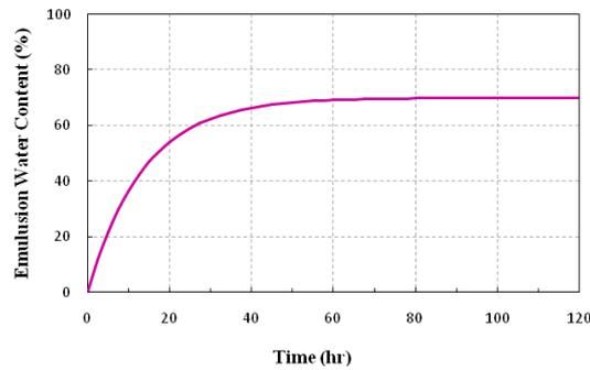
Fig. 5: The change of water content in water-in-oil emulsion
