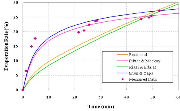
Fig. 3: Comparison of evaporation rates; wind speed = 5 m/s; temperature = 25 °C
