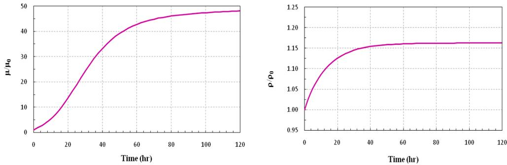
Fig. 7: The change of oil viscosity and density compared to their initial value
