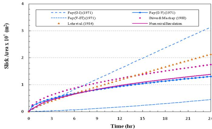
Fig. 1: Comparison between the dynamic model results and the empirical equations, test case 1
