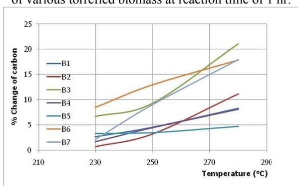
Fig. 3 Change in carbon content of various torrefied biomass as a result of torrefaction temperature.
