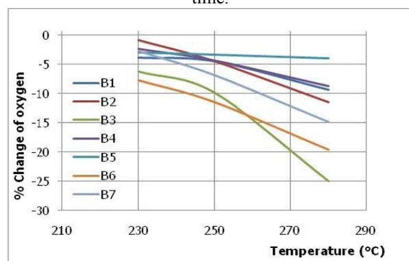
Fig. 6 Change in oxygen content of various torrefied biomass as a result of torrefaction temperature.
