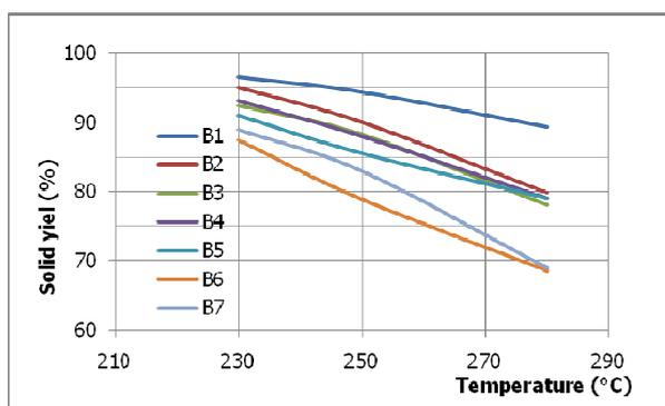
Fig. 1 Effect of torrefaction temperature on mass yield of various torrefied biomass at reaction time of 1 hr.
