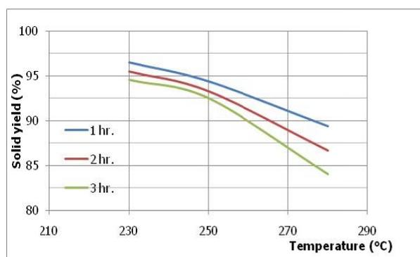
Fig. 2 Effect of torrefaction temperature on mass yield of torrefied biomass at various reaction time.
