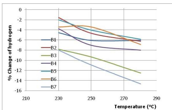
Fig. 5 Change in hydrogen content of various torrefied biomass as a result of torrefaction temperature.
