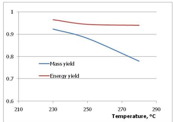
Fig. 10 Effect of torrefaction temperature on mass yield and energy yield of torrefied biomass
