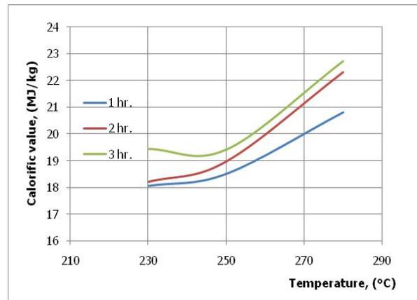
Fig. 8 Effect of torrefaction temperature on calorific value of torrefied biomass.
