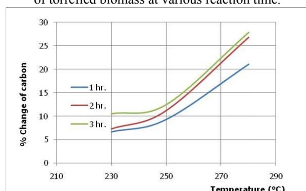
Fig. 4 Change in carbon content of torrefied biomass as a result of torrefaction temperature at different reaction time.
