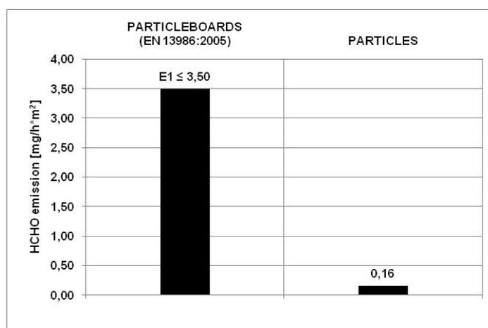
Fig. 4: Formaldehyde emission from E1-class particleboard permitted by EN 13986:2005 standard [11] and from absolutely dry pine particles contained in particleboard of density  $650 \text{ kg/m}^3$  and thickness 16 mm.
