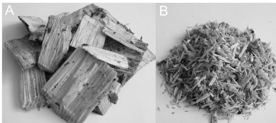
Fig. 1: Wood materials: A – chips, B – particles.
