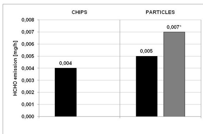
Fig. 3: Formaldehyde emission from wood at the beginning of processing chain – with respect 125 g of absolutely dry material (\*re-calculated to particleboard of density  $650 \text{ kg/m}^3$  and thickness 16 mm).
