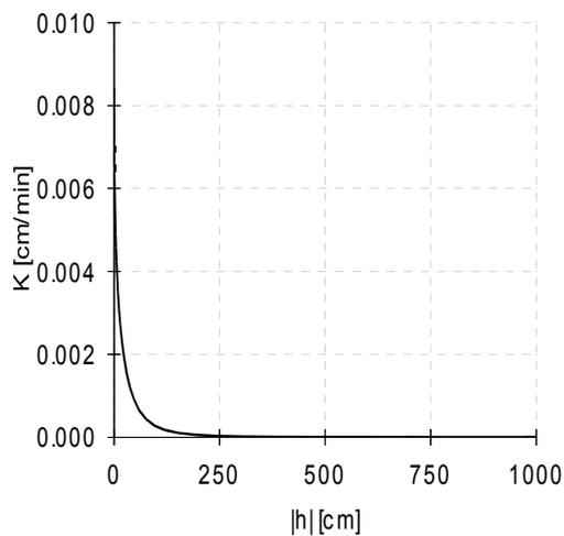
Fig. 8: Relative between hydraulic conductivity & matrix
