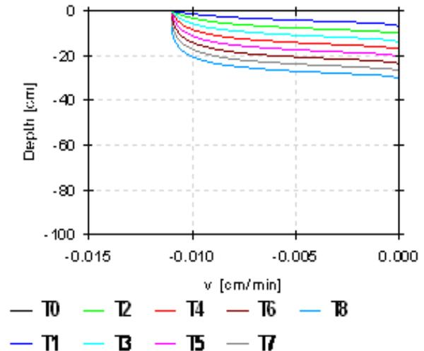
Fig. 7: Variations of hydraulic conductivity to depth in different periods
