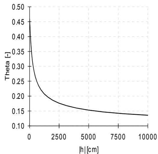
Fig. 9: Soil moisture characteristic curve
