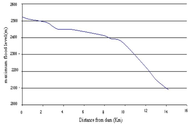
Fig. 3: Changing the maximum flood level at the down of the Bidakan barrier
