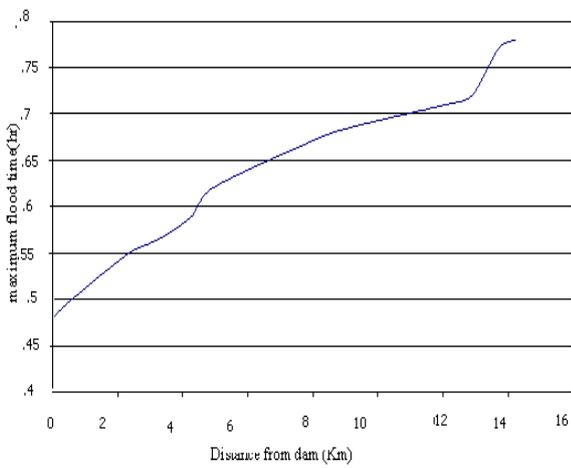
Fig. 4: Changing the maximum flood time at the down of the Bidakan barrier
