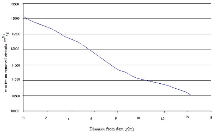
Fig. 2: Changing the maximum removal circuits at the down of the Bidakan barrier
