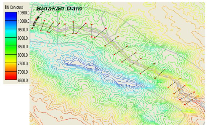
Fig. 5: Topographic lines and cross-section at the down of the Bidakan barrier before operating the model.
