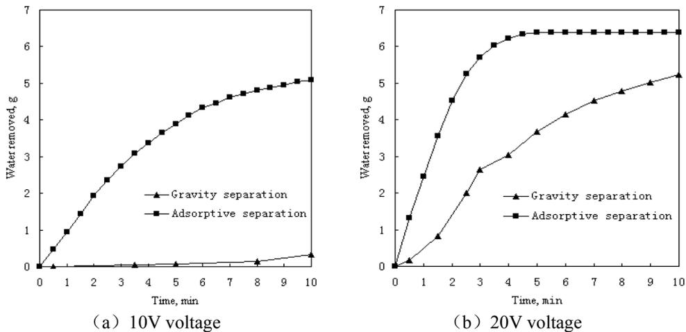
Fig. 2 Variation of water removed in EDW process of sludge (Filter cloth 0.4mm thick)
