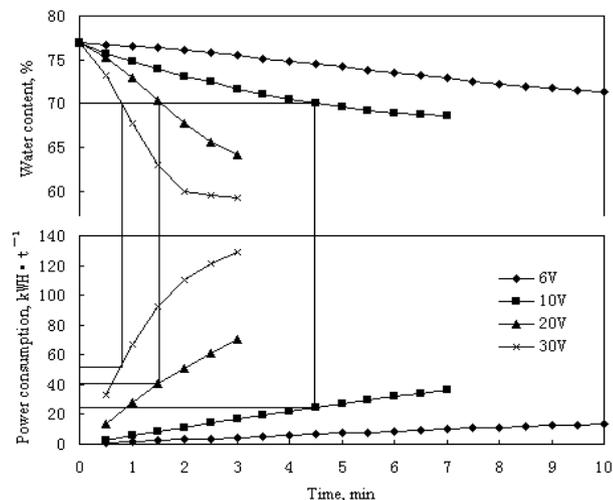
Fig. 5 Variations of water content and power consumption in adsorptive EDW
