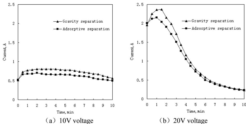
Fig. 3 Variation of current in EDW process of sludge (Filter cloth 0.4mm thick)
