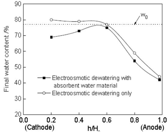
Fig. 4 Final water content distribution combined with absorbent water materials under constant voltage
