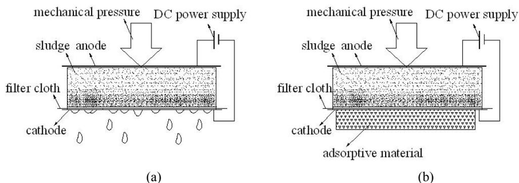
Fig. 1 The schematic of EDW using (a) gravity separation and (b) adsorption separation
