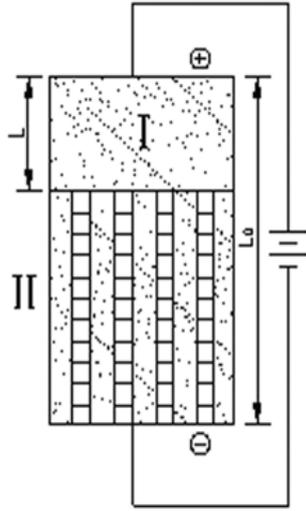
Fig. 6: Schematic diagram of electroosmotic dewatering model of sludge cake
