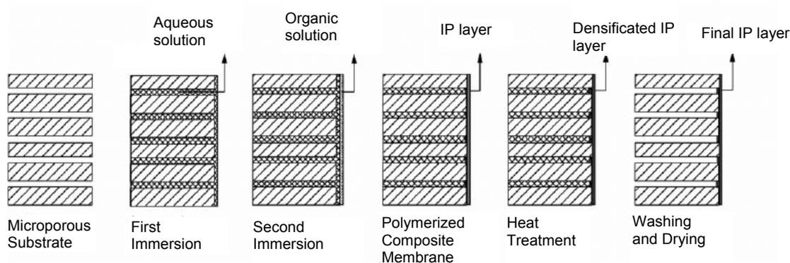
Fig.1: Schematic diagrams of the preparation process of TFC membrane by conventional IP technique
