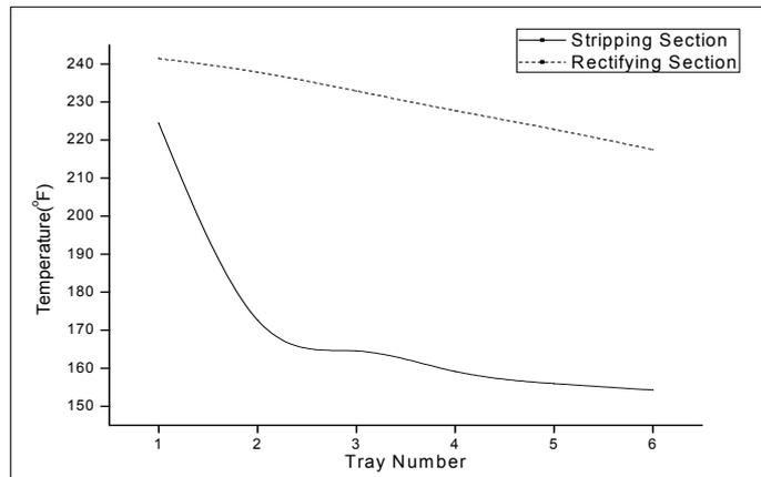
Fig. 1: HITDC stage temperature profiles (in this figure, stage numbering in both the sections is started from bottom up).
