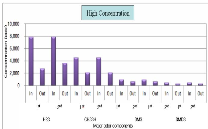
Fig .3. Tendency of odor removal with liquid spraying in high con-centration
