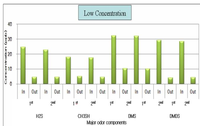
Fig. 2. Tendency of odor removal with liquid spraying in low concentration
