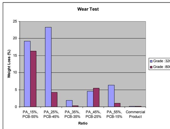
Figure 10: Wear result for different composition
