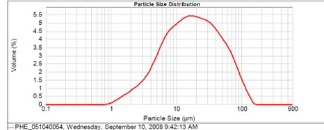
Figure 5: Particle size distribution of phenolic
