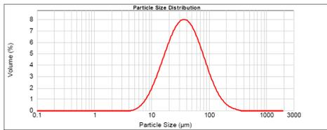
Figure 2: Particle size distribution of aluminum
