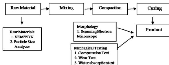
Figure 1: Flow chart of the raw material process
