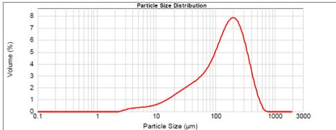
Figure 4: Particle size distribution of PCB
