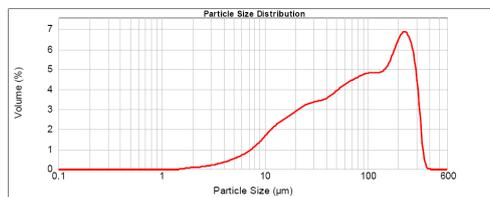
Figure 6: Particle size distribution of the brake pad mixture
