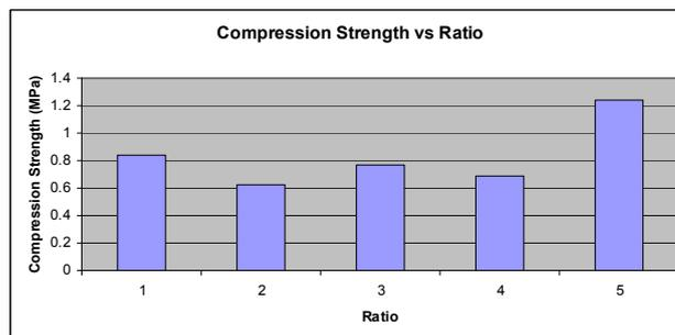
Figure 9: Compression Result for different composition
