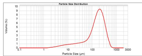
Figure 3: Particle size distribution of palm ash
