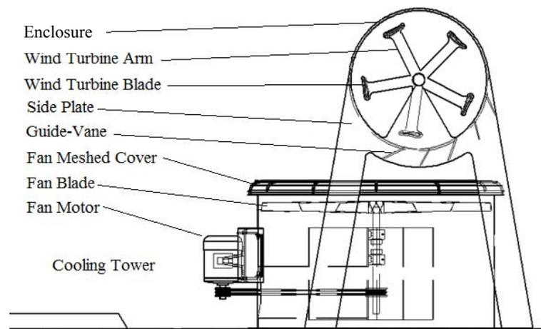
Fig. 2: Design arrangement of wind energy recovery system.
