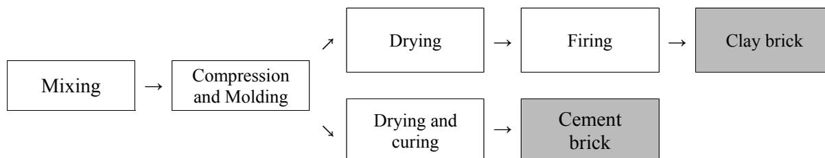
Fig. 2 : Manufacturing process of cement and clay brick
