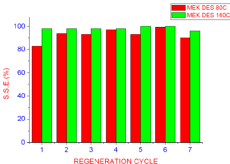
Figure 5 SSE of MEK spent adsorbent regenerated at different temperatures
