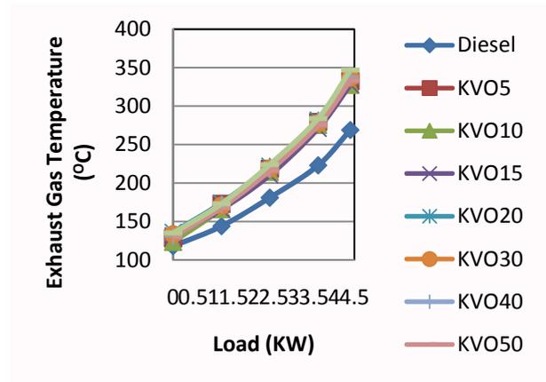
Figure 4 – Variation of exhaust gas temperature with load
