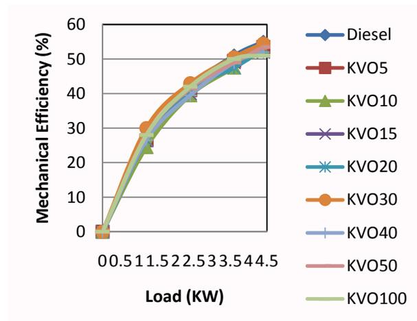
Figure 5 – Variation of mechanical efficiency with load
