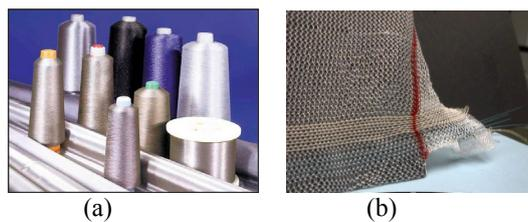
Fig. 4: Conductive yarns and fabric for e-textiles
