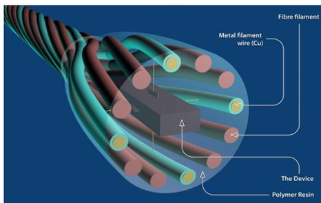
Fig. 5: Conductive yarn containing the device
