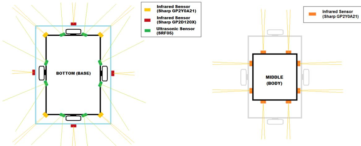
Fig. 5: Robot base and middle part sensor placement
