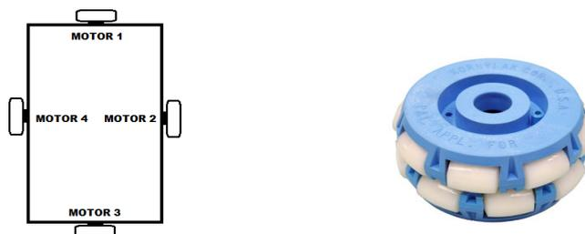
Fig. 2: Rectangular Wheel Configuration and Wheel Type
