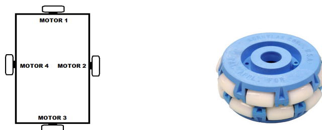
Fig. 2: Rectangular Wheel Configuration and Wheel Type
