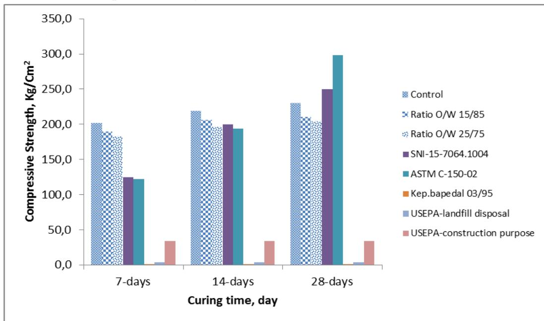
Fig. 2: Compressive Strength againts Curing Time
