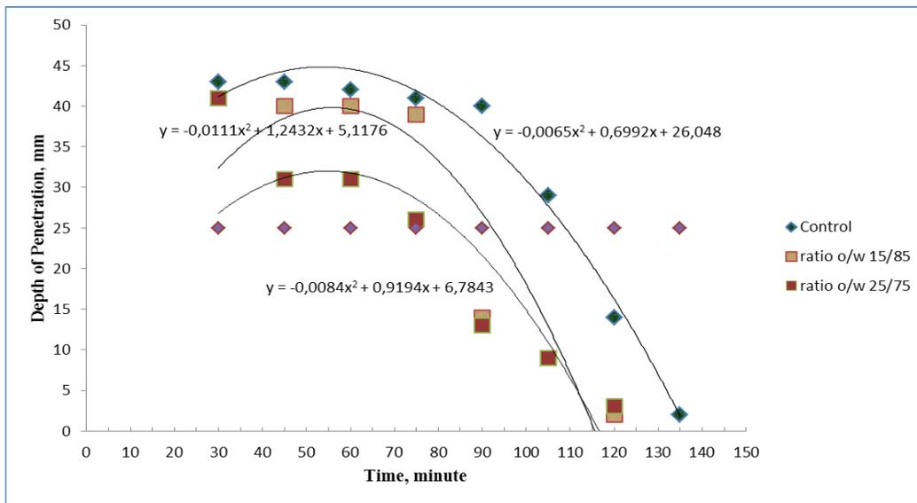
Fig. 1: Portland Composite Cement Depth of Penetration againsts Initial Setting Time
