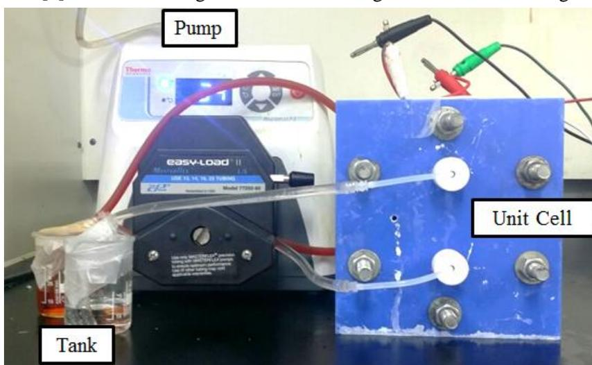
Fig. 2: ZBB cell experiment (active area: 6cm<sup>2</sup>, current density: 10mA/cm<sup>2</sup>).
