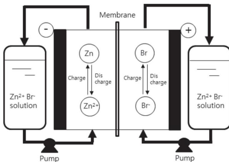
Fig. 1: Concept of the Zinc Bromine flow battery (ZBB).
