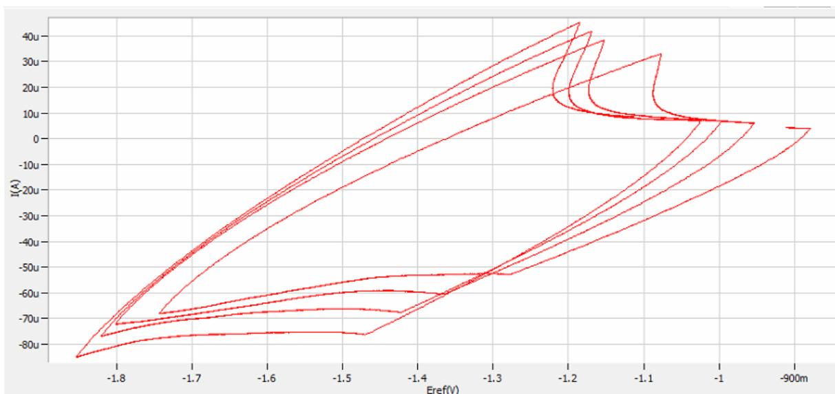
Fig. 1: Cyclic voltammogram of chromocene dissolved in N-methyle-2-pyrrolidinone (from 1<sup>st</sup> cycle to 4<sup>th</sup> cycle) vs. SCE electrode
