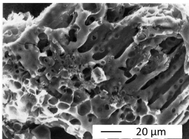
Fig. 3: SEM image of 750 °C cypress char (with PSK ash water-solution by 1:1, carbonized in N<sub>2</sub> stream)
