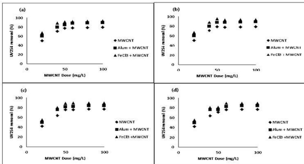
Fig. 2: Removal of UV<sub>254</sub> by MWCNTs and combined coagulation using jar test for (a) winter, (b) spring, (c) fall, and (d) summer. Optimum coagulant dose = 50 mg /l.
