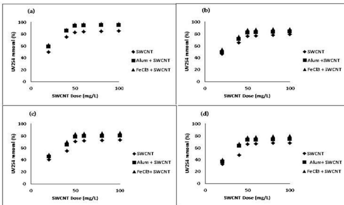
Fig. 1: Removal of UV<sub>254</sub> by SWCNTs and combined coagulation using jar test from (a) winter, (b) spring, (c) fall, and (d) summer. Optimum coagulant dose = 50 mg /l.
