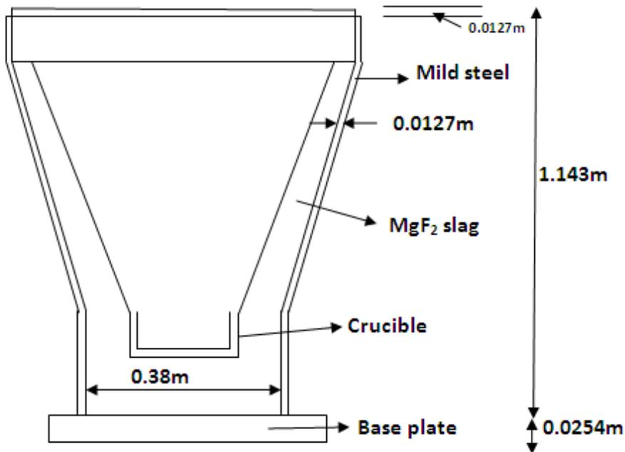
Fig.1: Geometry of MTR reactor (not to scale)
