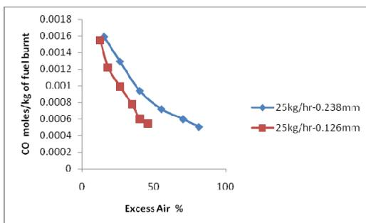
Fig 5: Effect of excess air on Carbon monoxide
