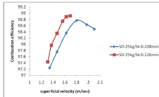
Fig 6: effect of superficial velocity on combustion efficiency
