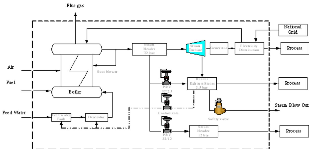
Fig. 1: System boundary for the analysis of the selected palm oil mill
