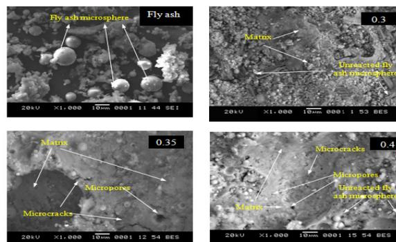
Fig. 4: SEM micrographs of the original fly ash and the synthesized geopolymers at activator/fly ash ratios of 0.30, 0.35, and 0.40 and a water glass/NaOH solution ratio of 1.0
