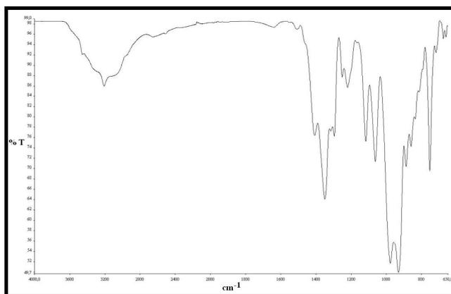
Fig. 5: FT-IR analysis of produced zinc borate (PG: 3% - IPA: 2 ml)
