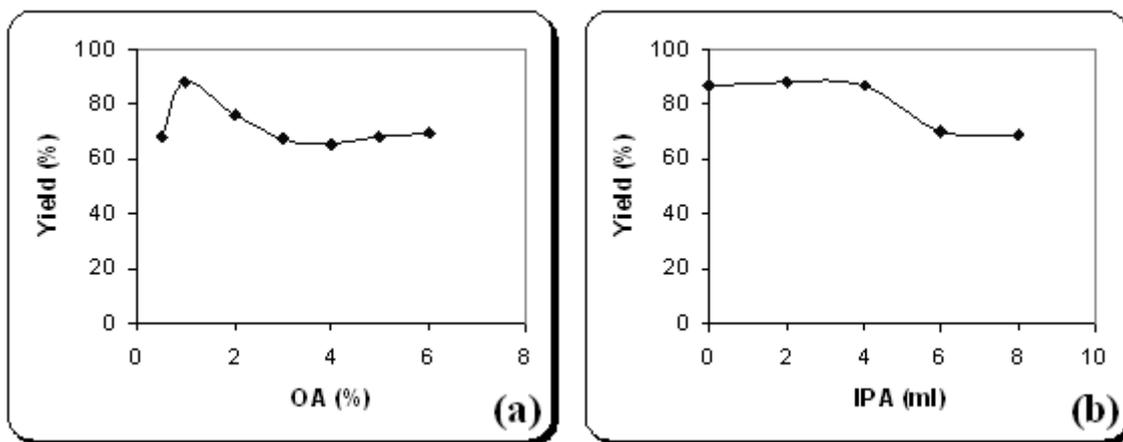
Fig. 3: Effect of oleic acid and isopropyl alcohol on yield: (a) OA, (b) IPA
