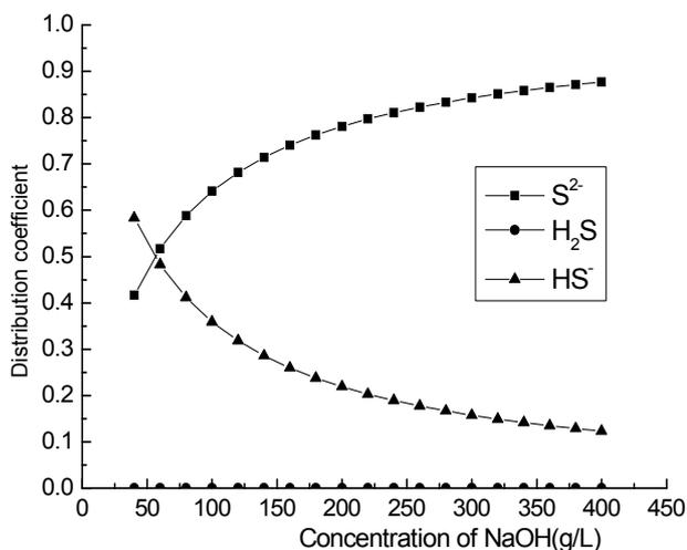
Figure 2. Distribution curve of Sulfur in alkali solution
