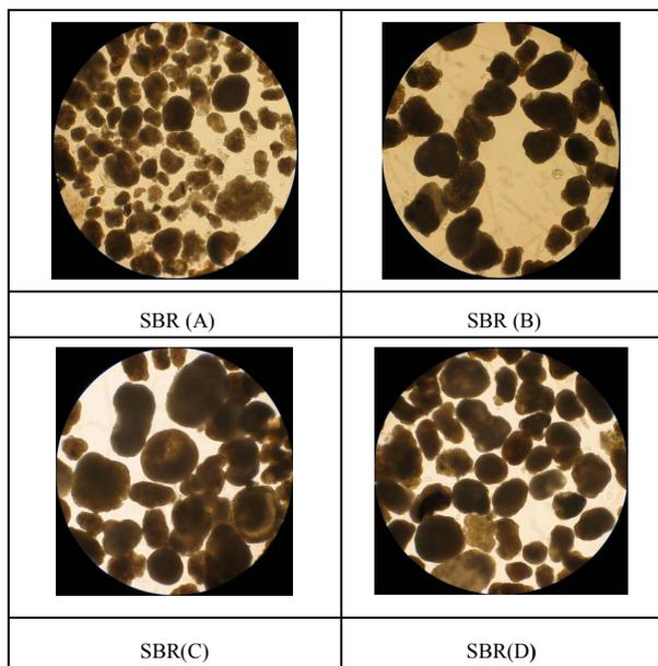
Figure 5. the mature aerobic granular sludge of different shear stress
