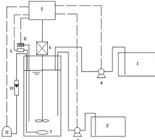
1. influent box 2. effluent box 3. effluent pump 4. influent pump 5. automatic control device 6. mechanical stirrer 7. diffuser 8. heating system 9. fluid level control 10. rotameter 11. air compressor
