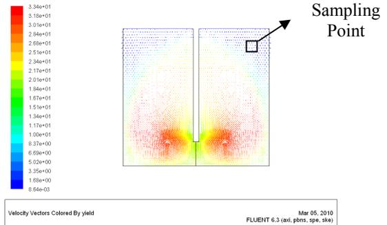
Figure 5. Velocity Vector of Yield (2.50x10-5m<sup>3</sup>/s AR, 2.50 SS).
