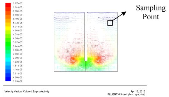
Figure 8. Velocity Vector of Productivity ( $2.50 \times 10^{-5}$  m<sup>3</sup>/s AR, 2.50 SS).
