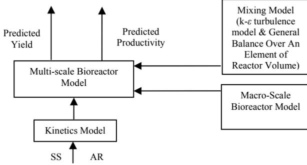
Figure 1. Schematic Diagram of Kinetics Multi-Scale Model.
