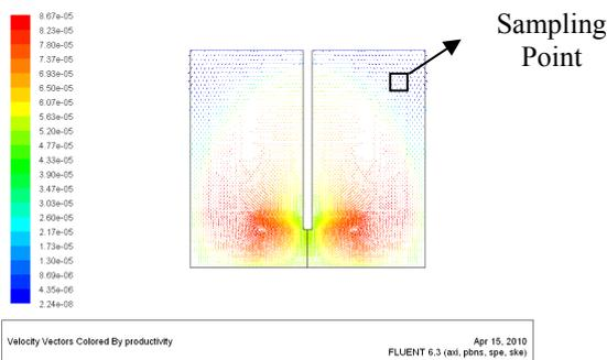
Figure 7. Velocity Vector of Productivity ( $2.08 \times 10^{-5}$  m<sup>3</sup>/s AR, 3.33 SS).
