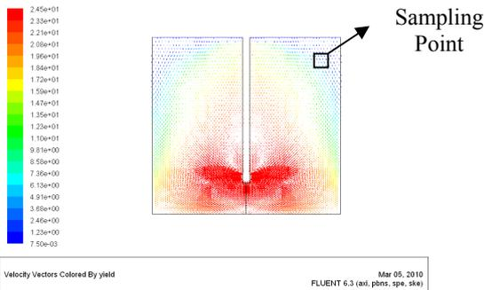
Figure 3. Velocity Vector of Yield (1.67x10-5m<sup>3</sup>/s AR, 4.17 SS).
