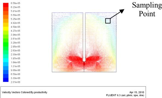
Figure 6. Velocity Vector of Productivity ( $1.67 \times 10^{-5}$  m<sup>3</sup>/s AR, 4.17 SS).
