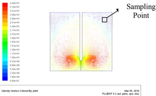
Figure 4. Velocity Vector of Yield (2.08x10-5m<sup>3</sup>/s AR, 3.33 SS).
