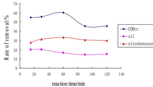
Fig.5 Removal rate of CODcr, nitrobenzene and oil with different reaction period
