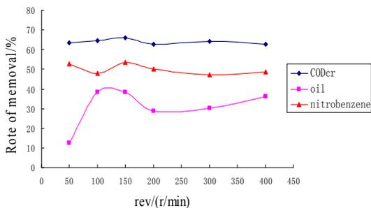
Fig.4 Removal rate of CODcr, nitrobenzene and oil with different rotational speed
