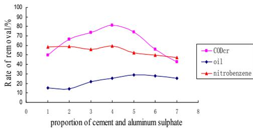
Fig.3 Removal rate of CODcr, nitrobenzene and oil with different proportion of cement to aluminum
