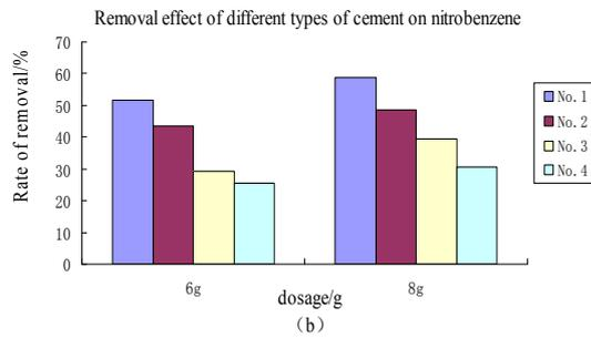
Figure 1. Removal effect of different of cement
