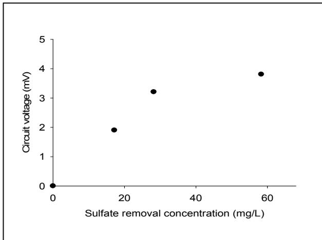
Figure 5. Relationship between sulfate removal and electricity generation.
