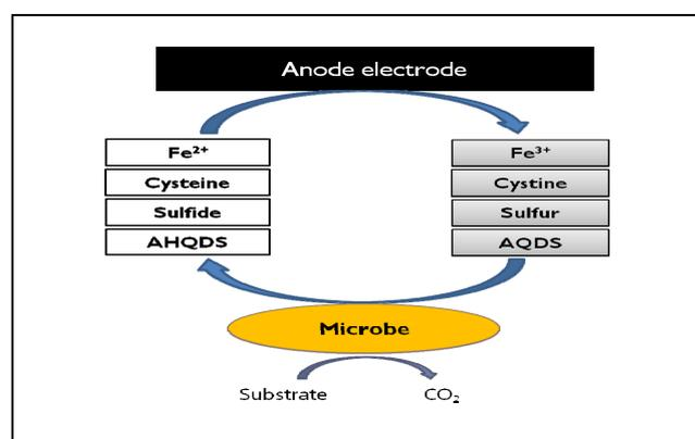
Figure 1. Electron shuttles in the MFC system [5].
