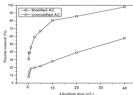
Figure 3. The effect of adsorbent dosage on the fluorine adsorption on MBC
