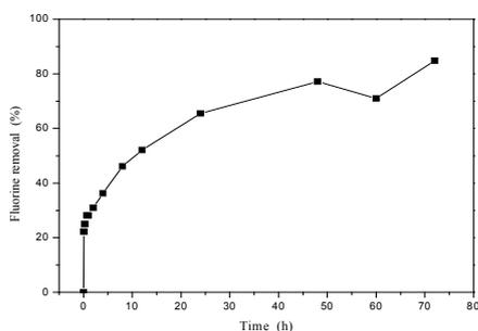
Figure 4. Kinetic of fluorine sorption from aqueous solution by MBC
