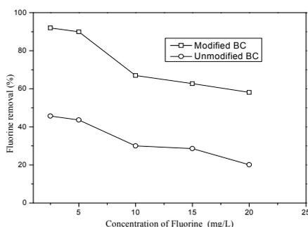
Figure 2. The effect of initial fluorine concentration on the fluorine removal by MBC.
