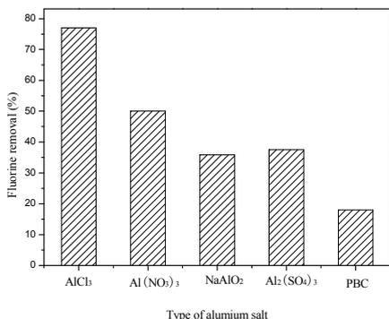
Figure 1. The effect of different alumium salts on the fluorine removal. (AlCl<sub>3</sub>: AlCl<sub>3</sub> modified plain bone char ;PBC: plain bone char)
